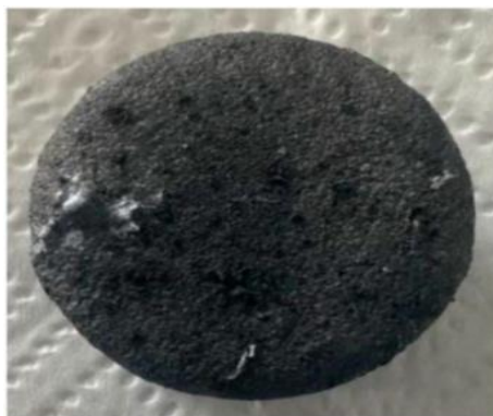
Fig. 2. Pb–Bi alloy after quenching.
